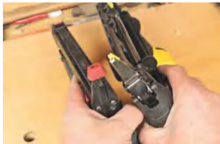
The Dewalt nose (right) is miniscule in comparison to a standard-nosed gun
